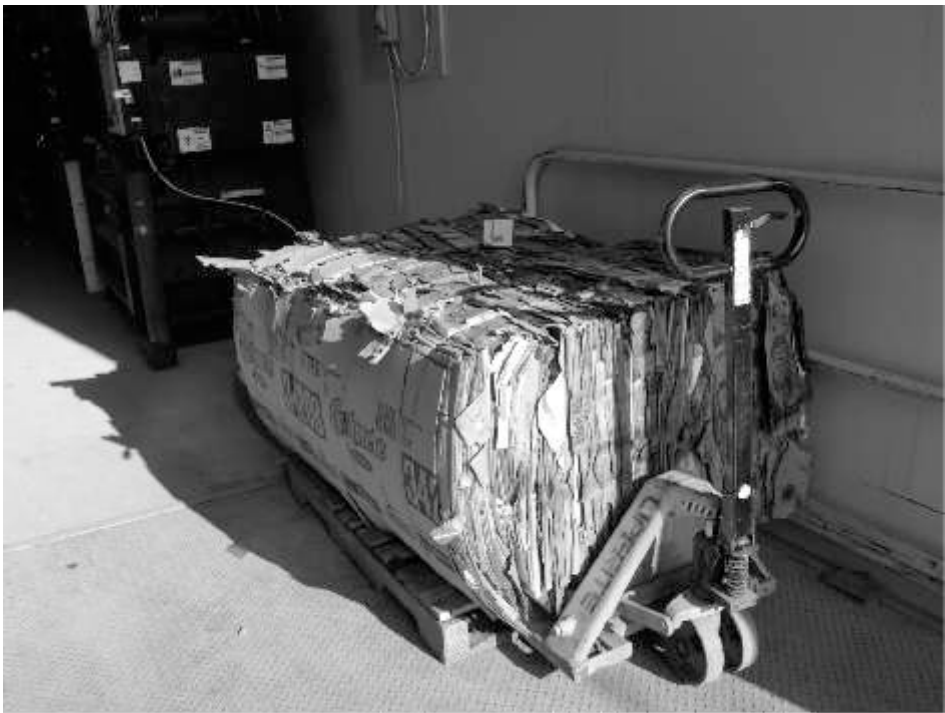
A week's worth of cardboard in the packaged bale weighing approximately 1 ton.
